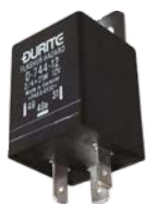
12V 1-6 x 21W hazard/flasher unit. Negative earth only. There is no bulb failure indication on this unit.
